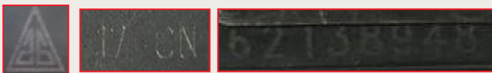
Marking for Factory 26, located in Chongjing, People's Republic of China (left); '17 CN' marking, indicating a manufacture date of 2017 (middle); eight-digit serial number (right).
